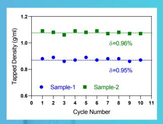
The 10 cycle measurements of two samples demonstrate the excellent **repeatability** (<1.0%) of the BeDensi T Pro Series.
