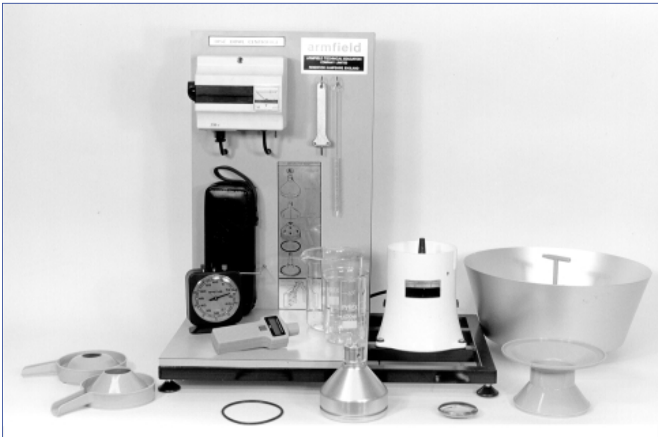
The Disc Bowl Centrifuge can easily be dismantled into its component parts
