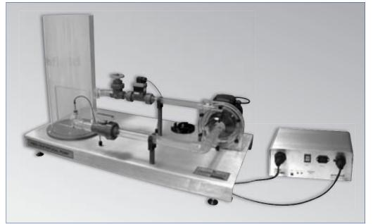
FM50 Centrifugal Pump Demonstration Unit shown with the IFD7 Interface Unit accessory.
