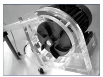
FM50 Centrifugal Pump with cover removed.
