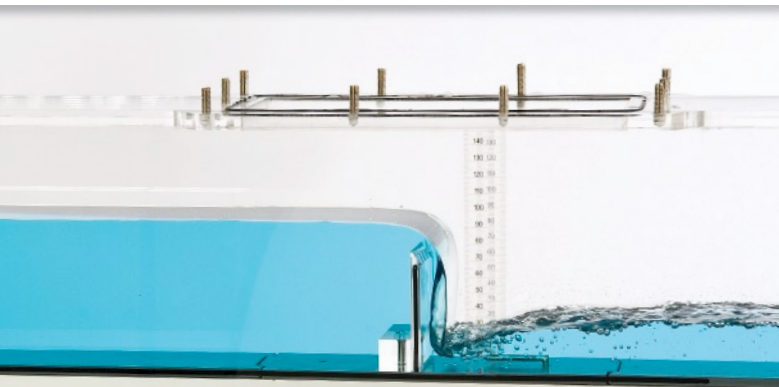
Flow over a sharp crested weir with the nappe (unventilated) clinging to the downstream face
