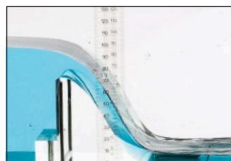
Smooth flow over an Ogee Weir.
