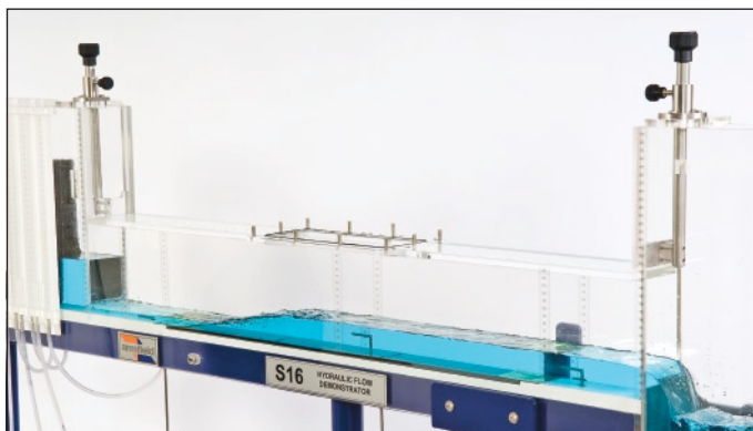
S16 configured as an open channel showing the hydraulic jump downstream of an undershot weir where energy is dissipated in the change from shallow super-critical flow to deeper sub-critical flow.
