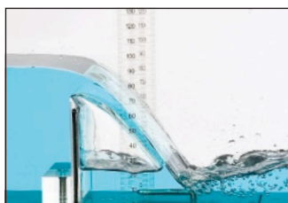
Flow over a Sharp Crested Weir with the nappe ventilated.
